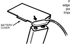
Remove the back cover. Place the edge of the cover between the battery posts and the battery. Pry up gently. Important: Do not pull the plastic wire connector to loosen it.
