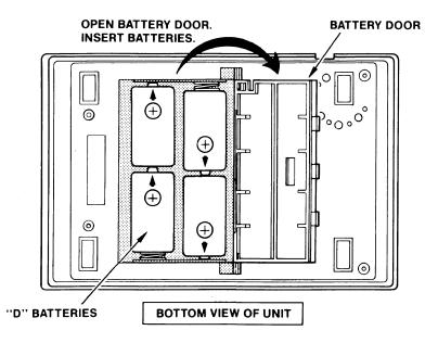
To insert batteries, open battery door and insert 4 "D" cell alkaline batteries in the order and direction shown. Close battery door.
