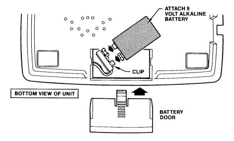
To insert battery, remove battery door on bottom of unit. Snap one 9-volt **alkaline** battery to the clip inside the compartment. (See illustration). Replace battery door.
