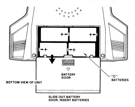
To install batteries, slide out battery door and insert 4 "C" cell alkaline batteries in order and direction as shown. Replace battery door.
