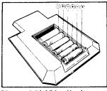
Place 6 "AA" batteries as shown in diagram. Do not reverse the direction.
